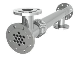
The K series heat exchanger is an all stainless steel shell and tube heat exchanger for industrial use. The product to be heated or cooled flows through the interior tubes. The media fluid flows through the surrounding shell. The K series is the ideal heat exchanger for steam to water applications such as CIP heating. Corrugated tubes are used to increase heat transfer rates which makes the K series much more efficient than normal smooth tube heat exchangers.
